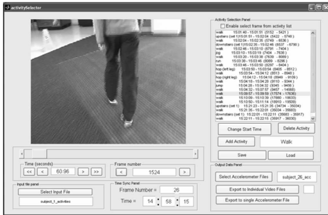
Fig. 2. GUI used to annotate the accelerometer data from the video record.
